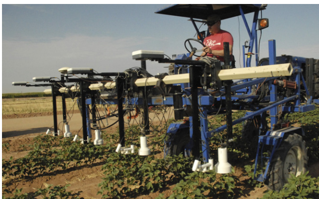
Fig. 1. High-clearance tractor in operation over young cotton plants at Maricopa, AZ. Replicated sets of sensors allow simultaneous measurement of canopy height, temperature, and spectral reflectance at three bandwidths. Real time kinematic GPS provides positional accuracy under 2 cm.
